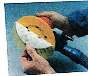
B Self-stick sandpaper has a controlled thickness of adhesive on the backside of the sanding disc. This type is preferred.
