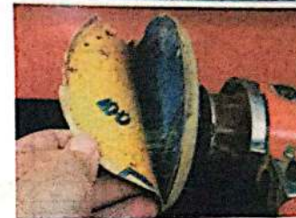
A Disc adhesive is an older method of holding sandpaper on the part, but the adhesive can contaminate the body surface.
